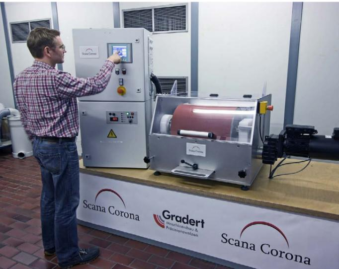
ensures even heat dissipation along the length and width of the electrode package. The air flowing in the discharge gap also ensures that energy-intensive surface streamers in the corona gap do not have a chance to form. Such surface streamers can cause local fusing on the surface of plastic sheeting that leads to significant damage.
