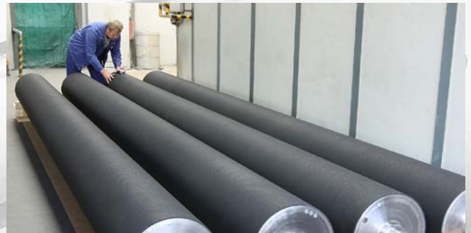
CFRP rubber roll, coating EPDM 70 shore, Ø 340 mm x 6100 mm
