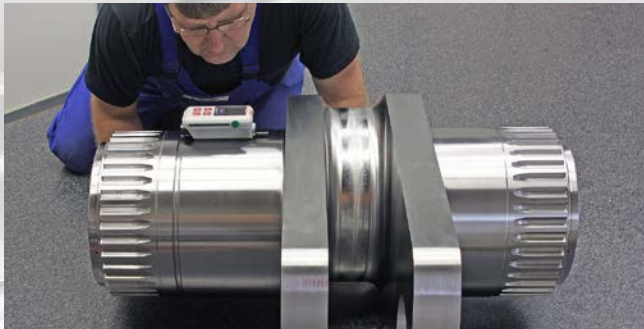
Crank shaft for punching machine, forging blank, 42 CrMo4
