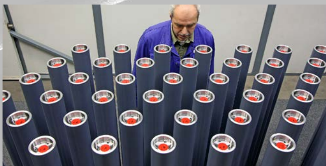
Oscillating roll for sheet-fed offset, Rilsan/PA11
