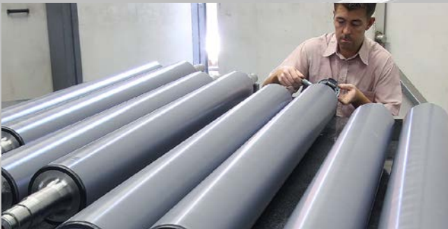
Oscillating roll, CFRP/Rilsan/PA11
