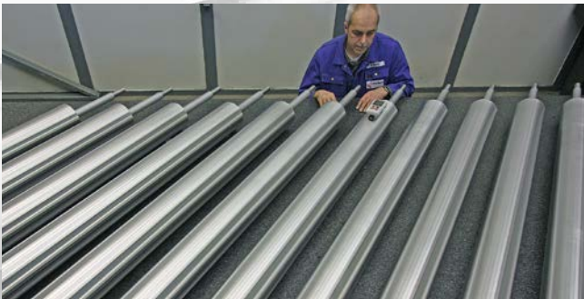
Aluminium guide roll, Ø 119 x 2800 mm, anodized
