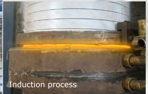
Induction hardening station for components up to 600 x 4000 mm
