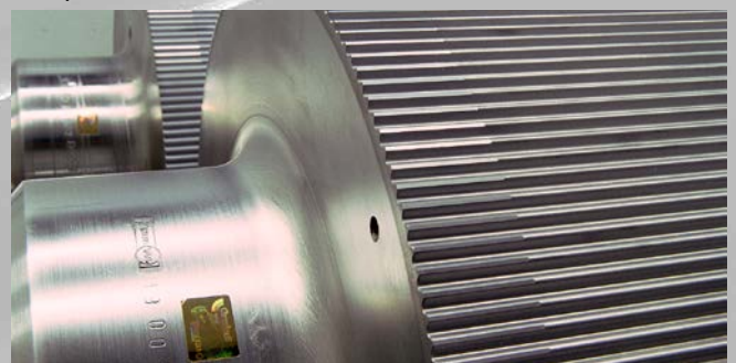
Corrugating rolls for a corrugated cardboard machine, tungsten carbide coating
