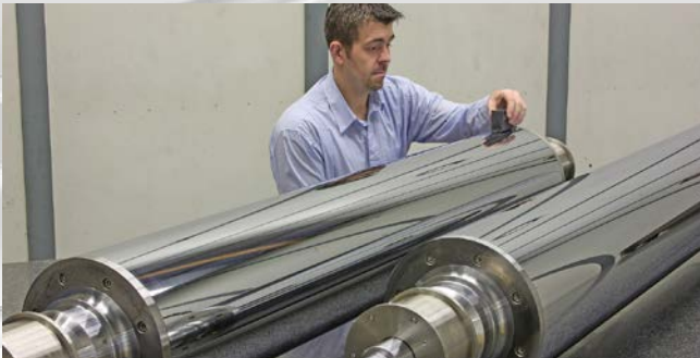
Precision roll, chrome, concentricity 0,002 mm, cylinder form 0,002 mm, high accuracy grinded
