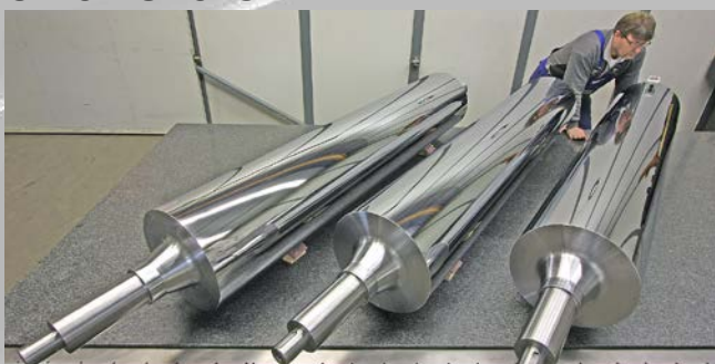
Chrome-plated cylinder, high gloss polished, Rz 0,05 µm
