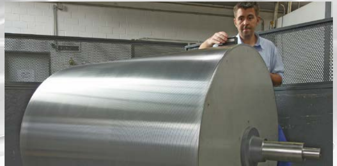
Cooling roll DW, creasing, Ø 1200 mm, chromed, 70 µm
