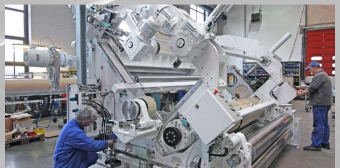
Single facer - corrugated cardboard machine during assembly
