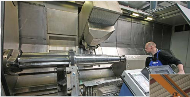
Millturn of a decoiler shaft on a Millturn M 120
