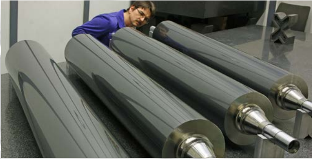
Ceramic cooling roll, concentricity 0,002 mm, cylinder form 0,002 mm
