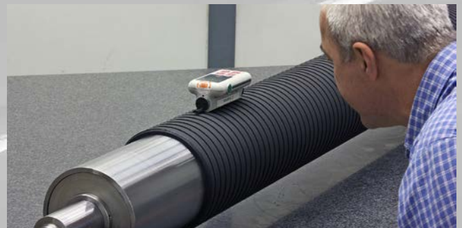
Spreader roll with special profiling, Neoprene 80 shore
