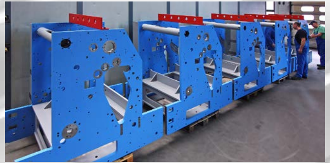
Printing units frame works
