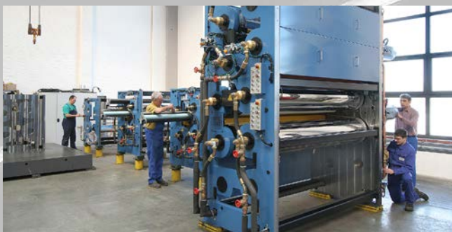
Cooling calender during assembly
