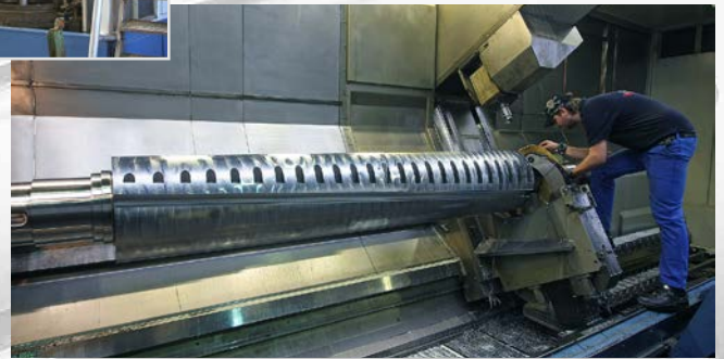
Manufacturing of a knife shaft, Ø 500 x 4000 mm
